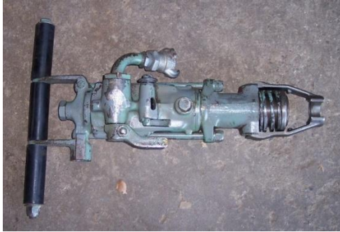
Figure 15 Gardner Denver GD 33-1 Rotary rock Drill
