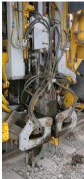
Figure 26 Vibrating tamping and lifting tool of tamper (Harsco 6700)
