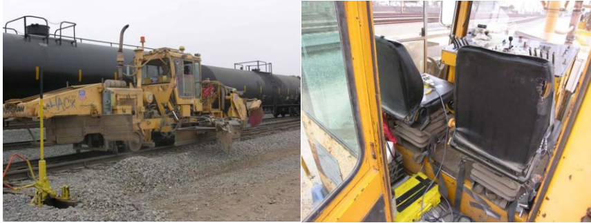
Figure 24 Ballast regulator and operator seat (Hasco 6700)
