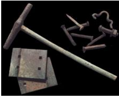
Figure 1 Spike driver, spikes, tie plates, clips, bolts and tong
