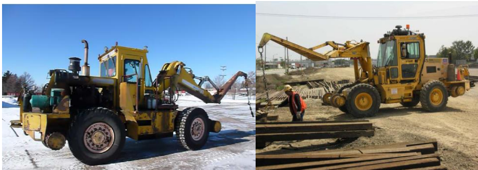
Figure 27 Tie crane vehicle (Speed Swing®)
