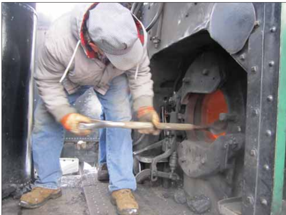
Brother Art shovels coal into the engine's firebox. It is important to keep the burning coal evenly spread to avoid cool spots.
