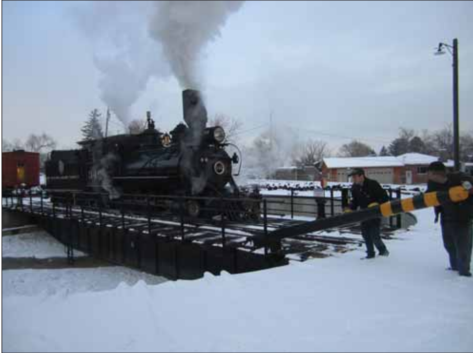
Volunteers use the manually-powered turntable to spin the No. 346 into position.
